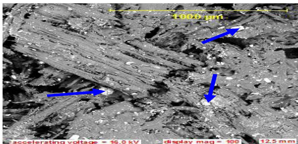
Figure 3: Micrograph of particle board, MCS spotted with blue arrow
