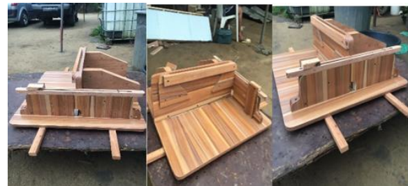
FIGURE 10. MJB READY FOR USE WITH CIRCULAR SAW MACHINE
