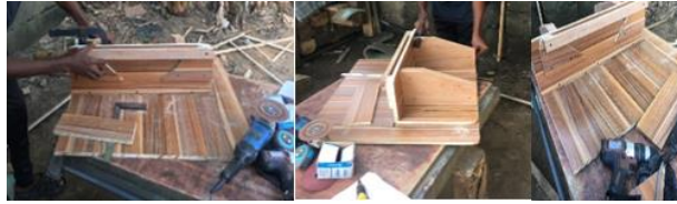
FIGURE 8. FABRICATION PROCESS OF THE MASTER JIG
